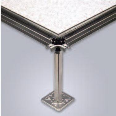
*Snap-Tite and Bolt-Tite Stringer* understructure system used primarily for gravity held panels with Integral Trim® edge in computer room or equipment rooms. This system allows for quick and easy access to the underfloor area.
